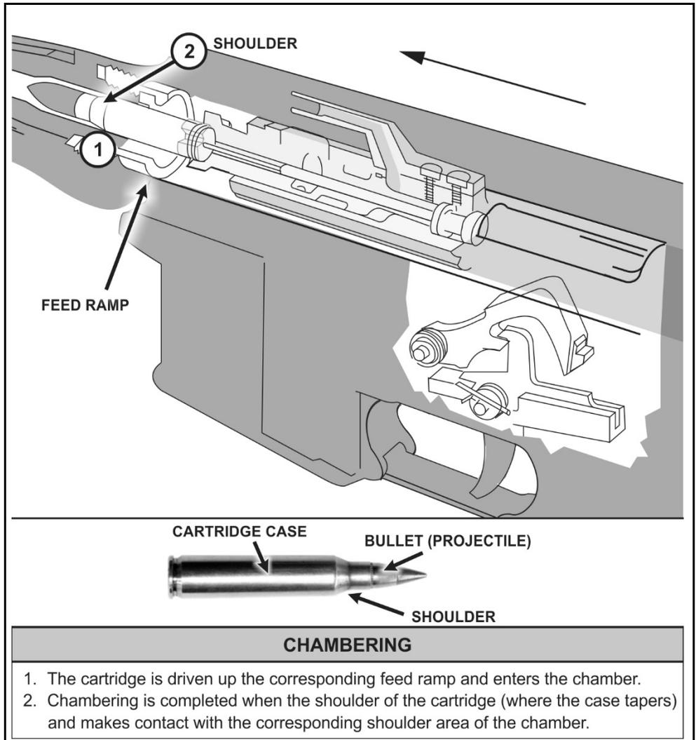
Figure 2-4. Chambering example
