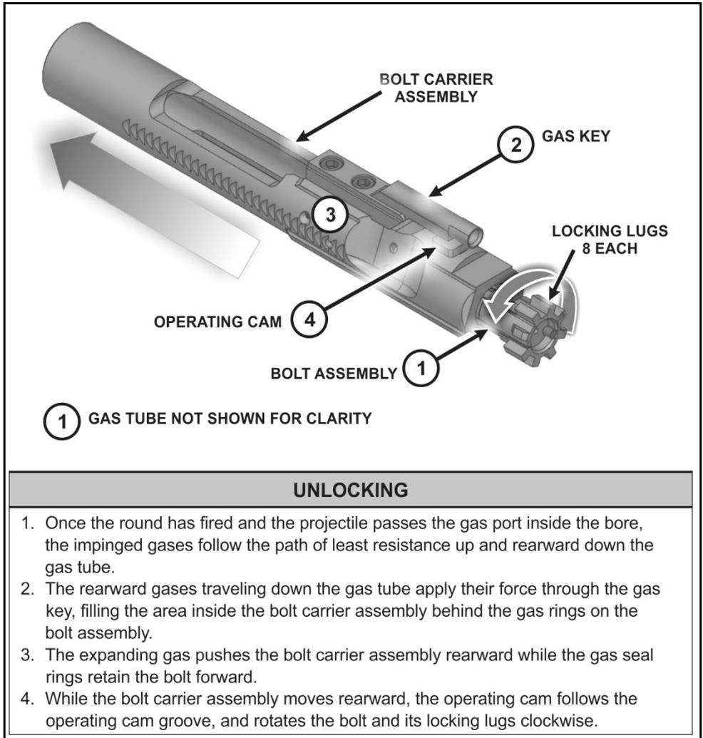
**Figure 2-7. Unlocking example**
