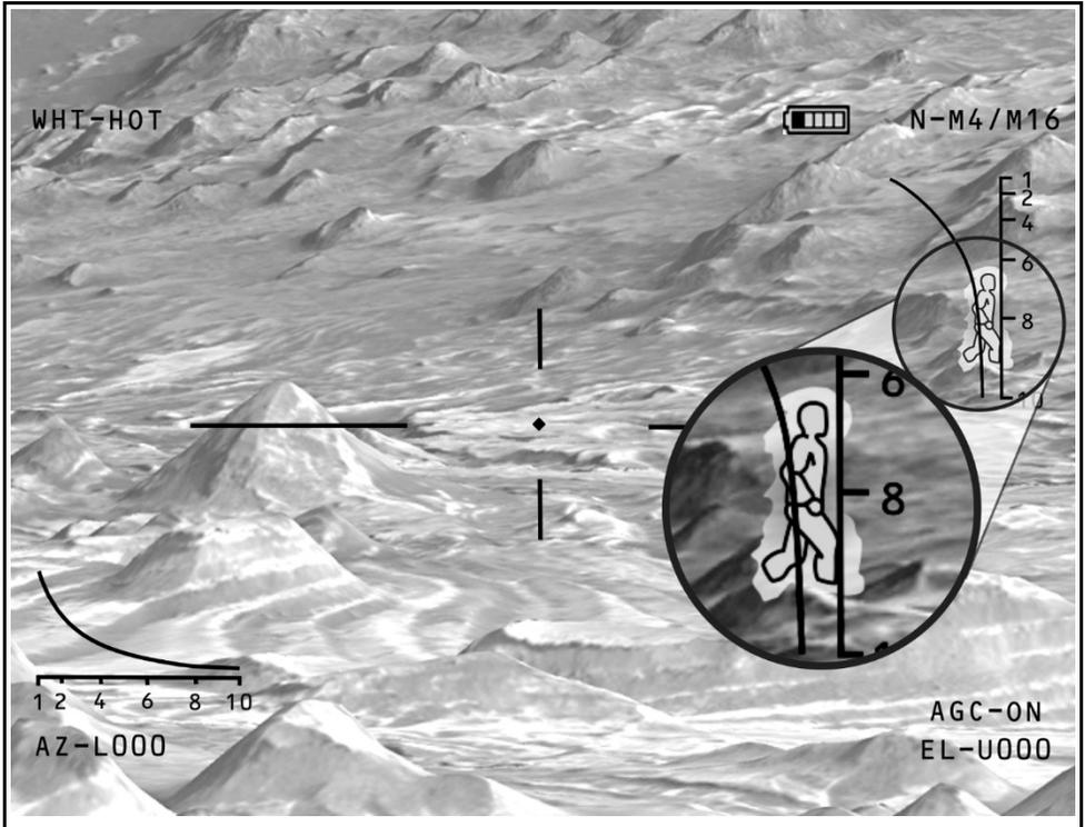
**Figure C-4. Reticle relationship using a stadiametric reticle example**
