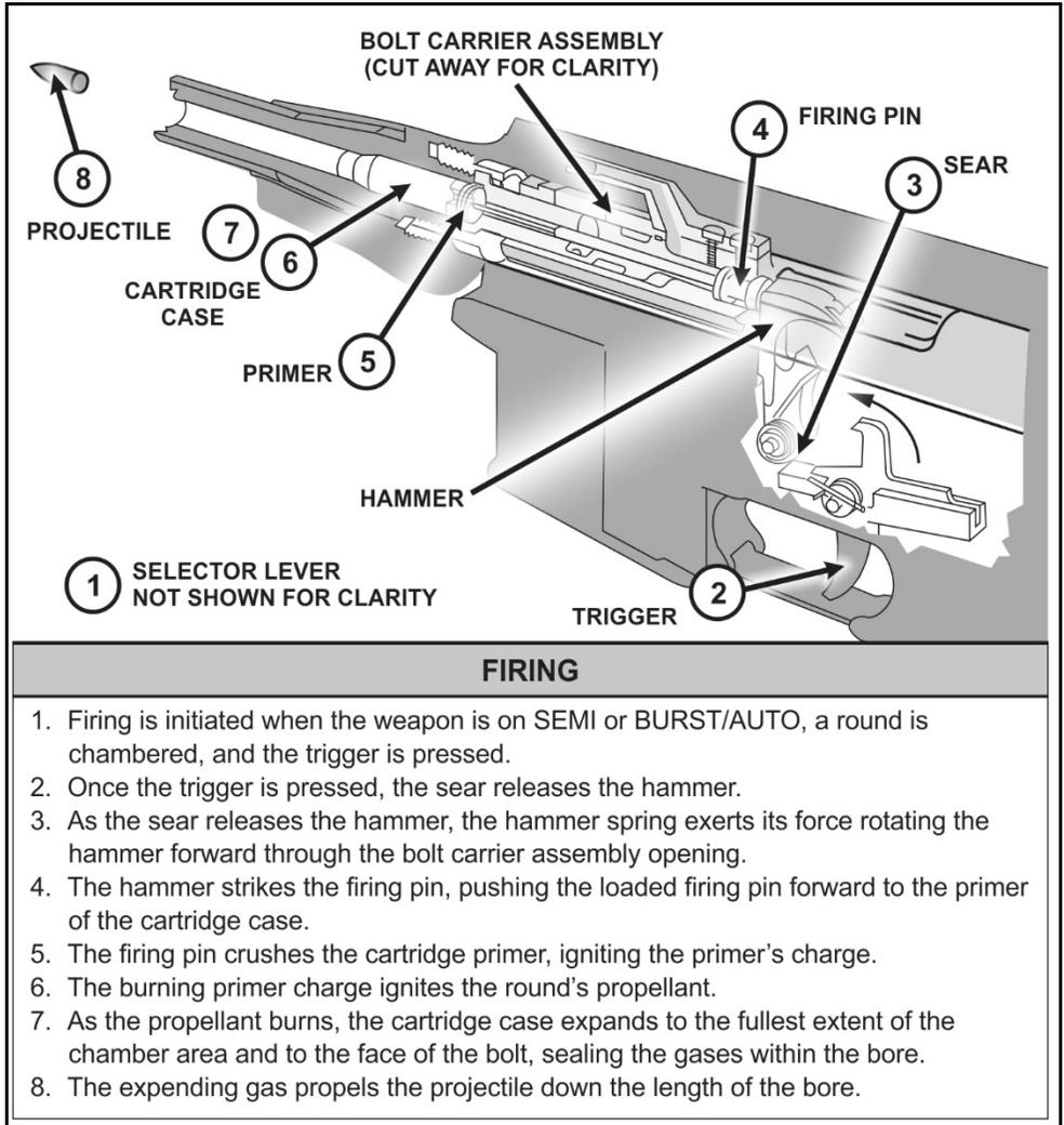
**Figure 2-6. Firing example**
