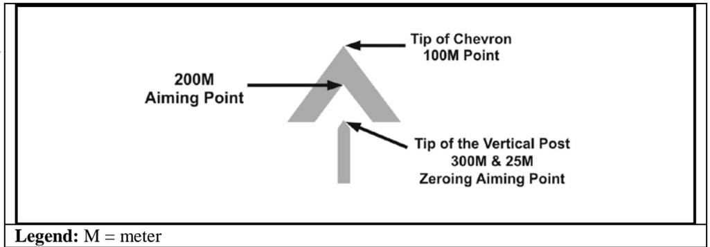
**Figure G-5. Advanced combat optical gunsight points of aim (100 to 300 meters)**
