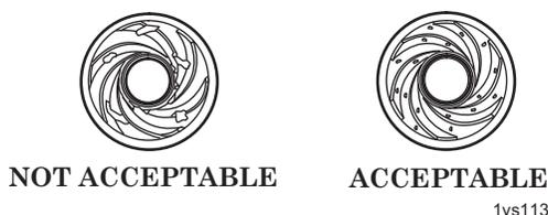
Figure 13. Bore Inspection.
